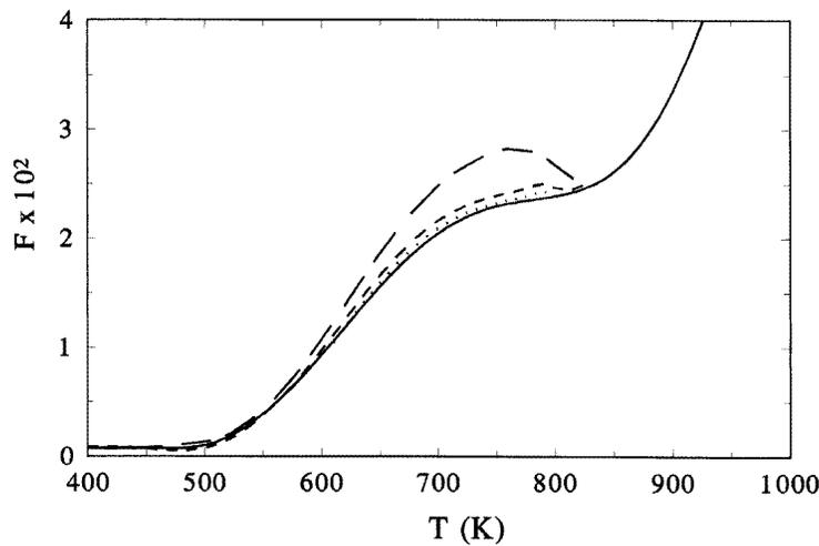
**Figure 2.** MDS spectra measured at  $\varepsilon_0 = 4.5 \times 10^{-5}$  for the set number 3 of samples (full line, 3; short dashed, 3'; long dashed, 3''). The dotted line represents the MDS spectrum for the irradiated sample under cover, but measured at  $\varepsilon_0 = 2 \times 10^{-5}$ .
