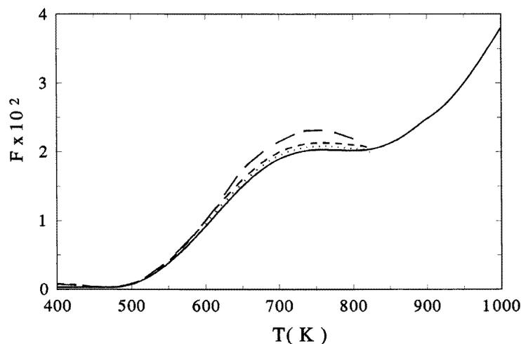
**Figure 3.** MDS spectra measured at  $\varepsilon_0 = 4.5 \times 10^{-5}$  for the set number 4 of samples (full line, 4; short dashed, 4'; long dashed, 4''). The dotted line represents the MDS spectrum for the irradiated sample under cover, but measured at  $\varepsilon_0 = 2 \times 10^{-5}$ .
