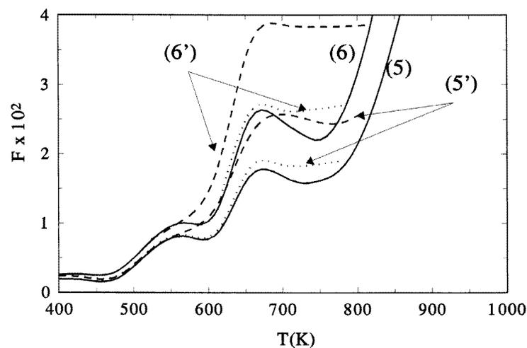
**Figure 4.** MDS spectra measured at  $\varepsilon_0 = 4.5 \times 10^{-5}$  for the cold-worked samples 5 and 6, unirradiated (full line) and irradiated (short-dashed line). Dotted lines represent the MDS spectra for the irradiated samples, but measured at  $\varepsilon_0 = 2 \times 10^{-5}$ .
